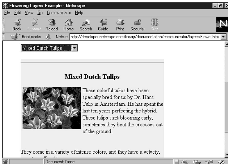
Figure 1.4. Using the <LAYER> tag and a form element, another set of text and graphics replaces the original picture.
